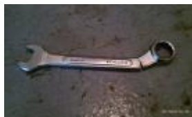
Gambar Kunci Ring patah
